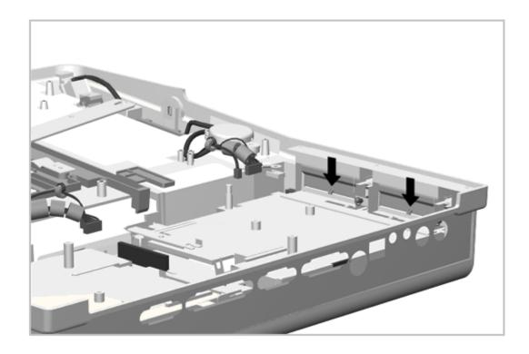
Figure 6-21. Installing the MultiBay Assembly
